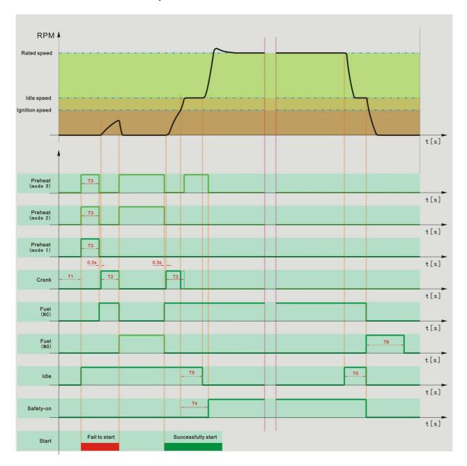
T1 – start delay T4 – safety-on delay T2 – crank time T5 – idle time
